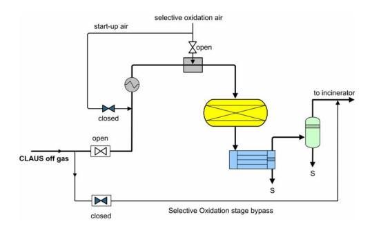
In case of a SUPERCLAUS<sup>®</sup> or EUROCLAUS<sup>®</sup> installation, oxygen concentration is designed to be just enough to convert H<sub>2</sub>S and keep the catalyst in an oxidized state. In the reactor outlet there should be just 0.5% to 1.0% oxygen present.
